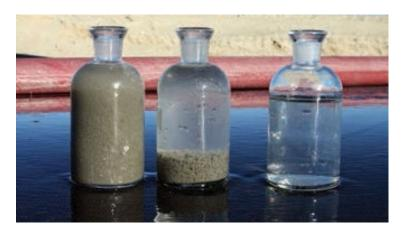
Sludge before (left) and after (right) treatment with **GEOTUBE**<sup>®</sup> dewatering technology
