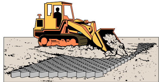
Figure 14 Fill Placement with Loader
